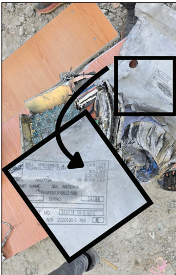
The missile fragments with Boulder's manufacturing information. Photo courtesy of Islamic Republic of Iran Broadcasting
